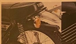
New silencer and muffler design cut down noise without cutting down power. Overthe-top exhaust and expansion chamber for better road clearance, less chance of burns.
