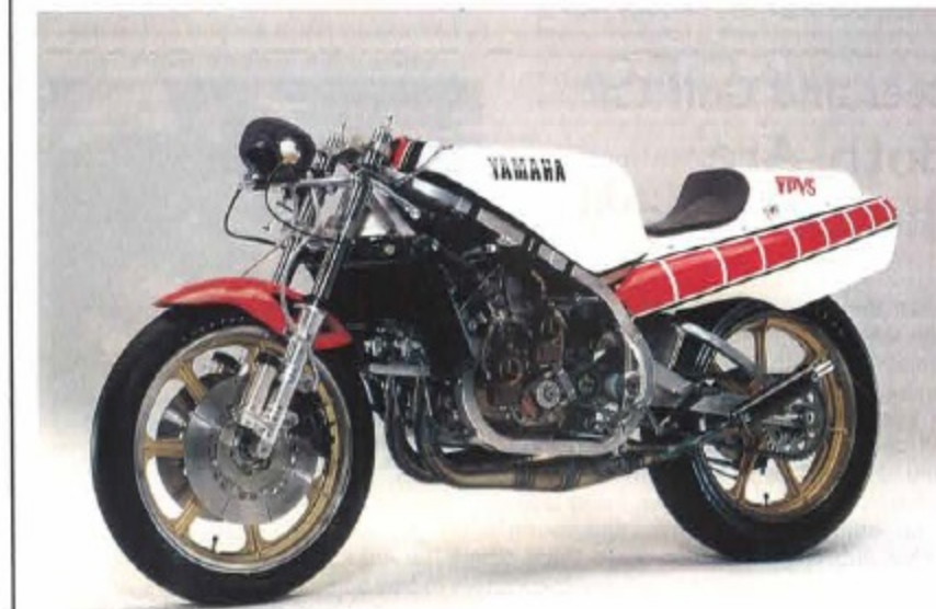
*Engine type: 2 stroke, water-cooled, YPVS, rotary disc valve, square 4 cylinders *Displacement: 499cc *Max. power output: — *Max. speed: — *Ignition: C.D.I. *Lubrication: Mixing (30 : 1) *Clutch: Dry multi-plate *Transmission: 6 speeds *Tire (Front): 3.25/4.00-18 (Rear): 4.30/6.30-18 *Suspension (Front): Telescopic (Rear): Swing arm (with Monocross system) *Brake (Front): Double disc (Rear): Single disc
