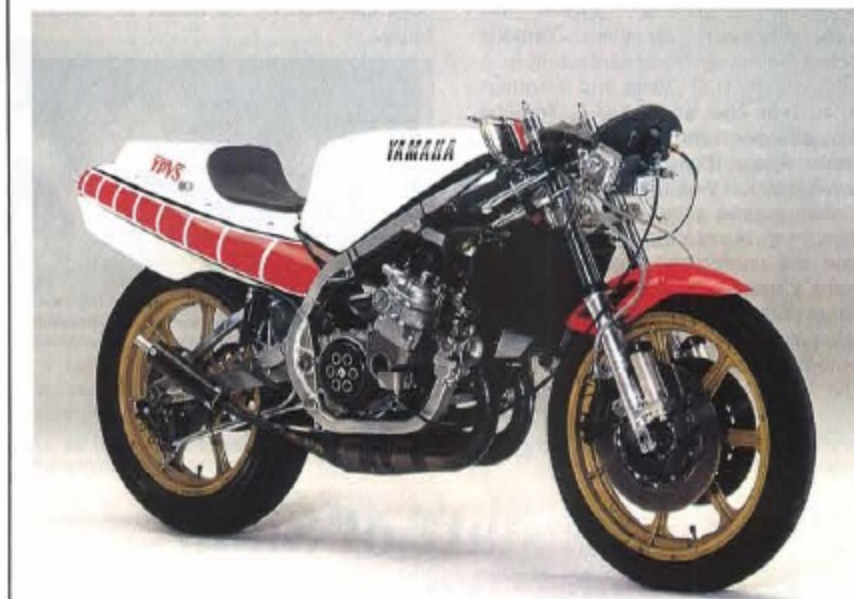
*Engine type: 2-stroke, water-cooled, YPVS, piston valve, parallel 4 cylinders *Displacement: 499cc *Max. power output: 120PS or more/10,500rpm *Max. speed: 270km/h or more *Ignition: C.D.I. *Lubrication: Mixing (30 : 1) *Clutch: Dry multi-plate *Transmission: 6 speeds *Tire (Front): 3.25/4.00-18 (Rear): 4.30/6.30-18 *Suspension (Front): Telescopic (Rear): Swing arm (with Monocross system) *Brake (Front): Double disc (Rear): Single disc *Weight: Less than 138kg
