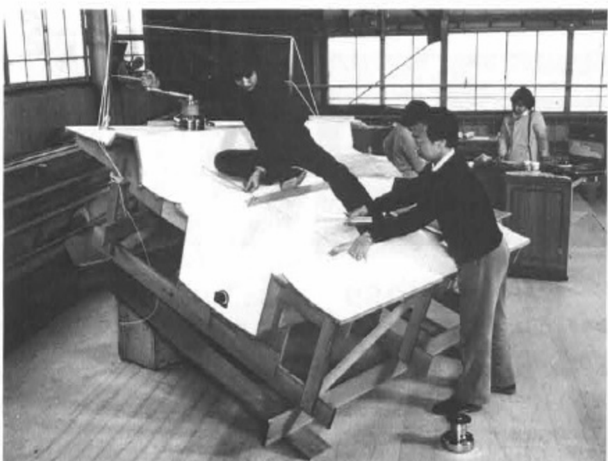
Full scale mock-up is used to make sure the sailboat has the best human engineering possible.
