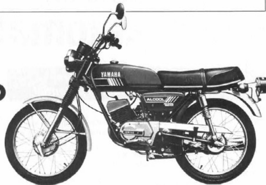
Yamaha RX125AL is the first 2-stroke 100% alcohol bike ever produced in the world. 6,000 machines will be produced per annum.
