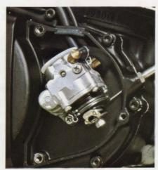
Continuously monitoring the rotational speed of the engine and the throttle opening, Autolube precisely controls the amount of oil, from a separate tank, to be mixed with the gasoline. This automatic gasoline and oil mixing system, which was developed by YAMAHA, improves engine operation by maintaining optimum performance under all riding conditions.
