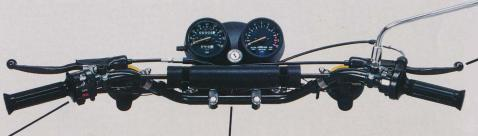
The Enduro MX has full instrumentation including speedometer and tachometer.
