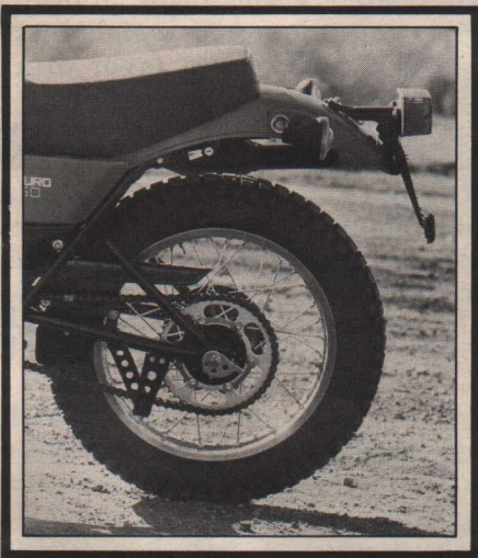
Lock to rear of seat pops saddle up to get to tool kit and oil tank. Luggage space measures eight inches behind seat.
