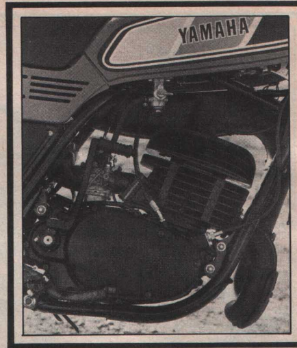
Side panels pop off. Battery and injection oil are behind left panel. Oil tank swivels out for easy filling. Right side cover is locked, has swivel dust protector. Tool kit and air filter access are behind it.
