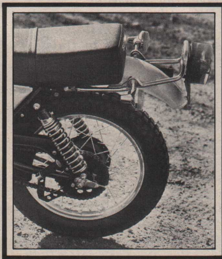
That's a helmet lock below seat. Turn signals can be flexed in any direction, best yet for the dirt.
