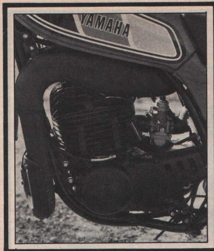
Side panels pop off. Battery and injection oil are behind left panel. Oil tank swivels out for easy filling. Right side cover is locked, has swivel dust protector. Tool kit and air filter access are behind it.
