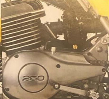
Torque Induction<sup>®</sup>, Yamaha's exclusive reed valve intake system, produces remarkable low speed torque. The large flywheel design of the TY 250's engine and the close-ratio five speed transmission also help it pull hard at low speeds.
