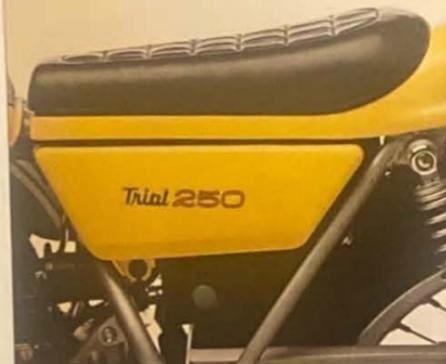
Slim trials saddle and a very narrow crankcase make for a comfortable riding position when you're up on the pegs. Every major component of the TY 250 has been designed specifically for trials.
