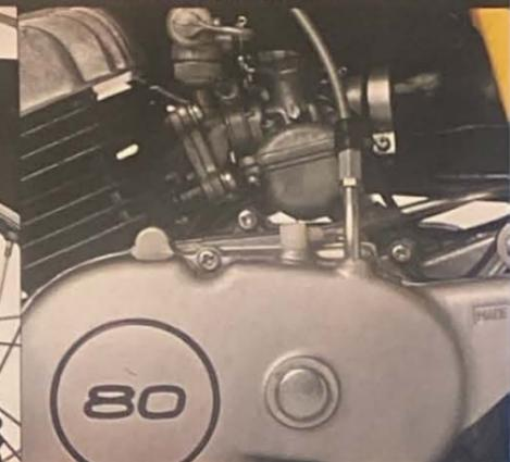
Torque Induction<sup>®</sup> helps the TY 80 generate more low speed torque by feeding the engine exactly the amount of fuel and air it needs. Large flywheel design also helps make for excellent low speed control.
