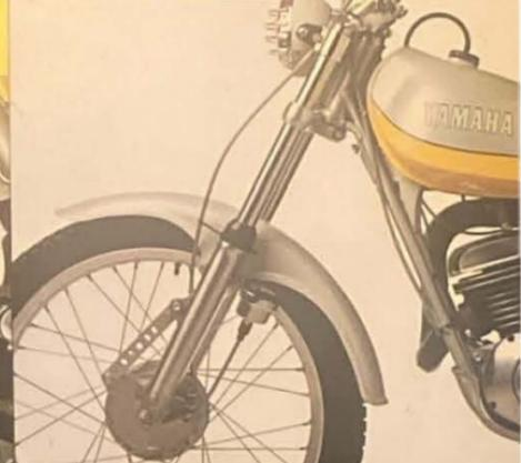
Trials front forks have extremely soft damping action. Lightweight speedo is mounted on fork. Hubs and rims are alloy. Fenders and gas tank are polypropylene. Even the Autolube<sup>®</sup> tank is lightweight nylon.
