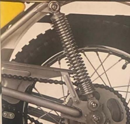
Special design rear shocks and front forks are long-travel units with soft damping characteristics to maintain control on rugged terrain. And to help the wheels ride up over high obstacles easily.
