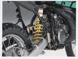
The DT's powerplant reveals the machine's close technological ties with our factory racers. The fuel/ air mix is fed directly into the crankcase through a TM28SS flat slide carburettor to give instant throttle response. Developed from our racing programme, the Yamaha Energy Induction System (YEIS) gives strong low and mid range torque.
