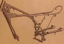
The frame for the TY250 is an extraspecial diamond type which has been constructed of slim, high-tensile-strength tubing to offer a more dynamic ability to withstand stresses and strains encountered from the roughest sections imaginable.
