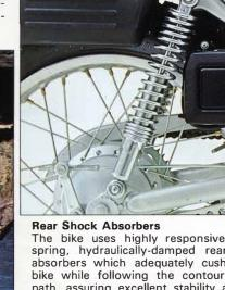
The bike uses highly responsive, outerspring, hydraulically-damped rear shock absorbers which adequately cushion the bike while following the contour of the path, assuring excellent stability and balance. Also, these shocks are adjustable in 5-steps so that the tension of the rear shocks can more accurately match that of the section to be ridden.
