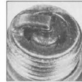
Incorrect burning: electrode is sooty or sometimes wet.
