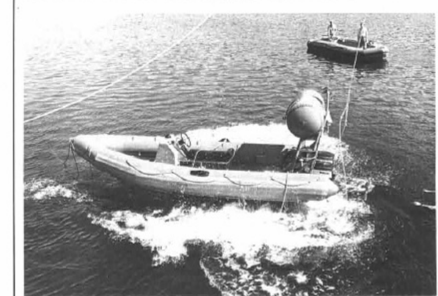
Great Britain: A capsized boat! A disaster? No, not quite. This is a test conducted by the staff of British Mitsui Yamaha on their special self-righting Yamaha outboards. They are completely watertight and incorporate a newly designed self-righting device. The test is a success. The boat has returned to its upright position. These special outboards have proven to be very useful for safe rescue operations on rough sea.
