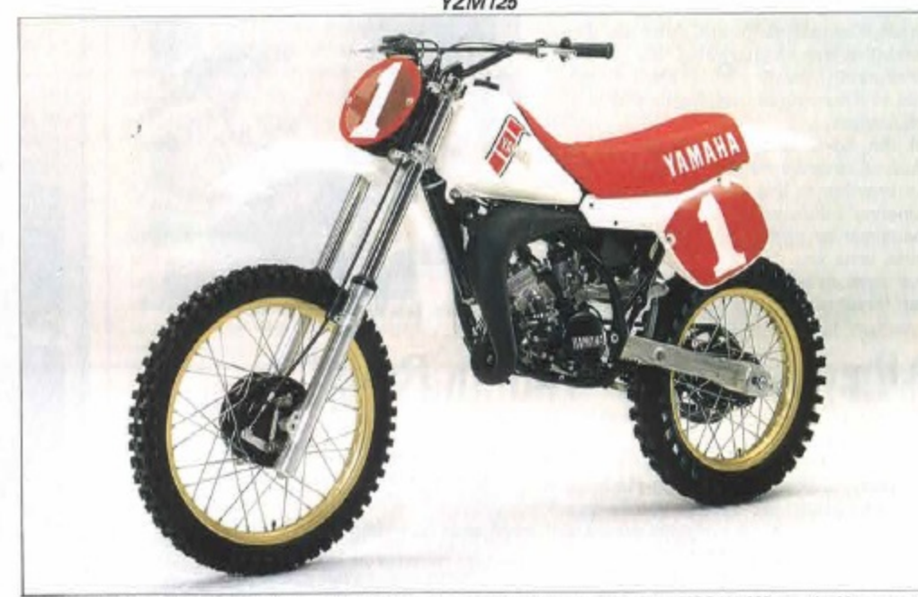
YZM125 *Engine: 2-stroke, water-cooled single *Displacement: 123cc *Max power output: Over 30PS/11,000rpm *Ignition system: C.D.I. *Lubrication system: Pre-mixing (20 : 1) *Transmission: 6-speed gearbox *Tire size (F): 3.00-21 (R): 4.00-18 *Brake (F): Drum (R): Drum *Suspension (F): Telescopic fork (air damper plus coil spring) (R): Swing arm (with Mono-cross unit) *Fuel tank capacity: 7.0 lit *Clutch: Wet multiplate
