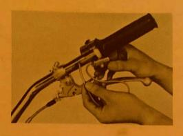
15) As shown in the photo to the right, thread the kill switch lead wire through the hole under the right handlebar.
