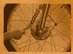
8) Install the front wheel on the front forks.
