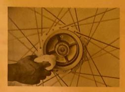
7) Wipe off any dust on the brake shoe linings and drum with a clean cloth.
