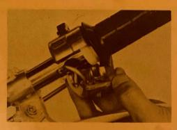
16) Align the locating pin (attached to the lower side of the throttle grip housing) with the hole in the handlebar.
