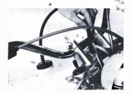
24) Connect the air breather pipe to the fuel tank cap, and thread it through the hole located in front of the steering upper crown.
