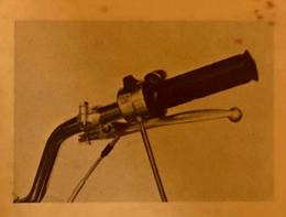
17) Bolt the upper and lower throttle housing together, and check the throttle grip for smooth action, then fully tighten the throttle housing securing screws.
