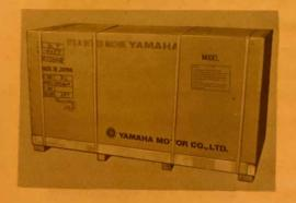
1) The TY250A is put in a cardboard crate. To unpack, cut plastic bands wound around the cardboard crate using a cutter, and then take it out. Lift the top off the crate by pulling it straight up with an assistant.
