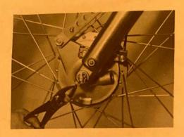
11) Lock the wheel shaft nut with the cotter pin.
