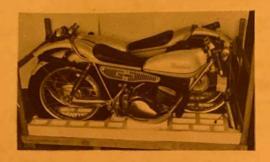
3) Take out the front fender which is placed between the rear wheel and the rear fender, and take out the front wheel.
