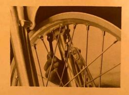
13) Insert the front fender between the front forks, and secure the front fender using 6 mm hex head bolts, spring washers and plain washers, for each.
