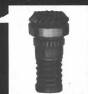
The newly designed shaft-drive system. The middle gear is built in the crankcase, reducing the total weight by 3kg, compared to a conventional system. The drive damper is also newly designed to improve the performance of the shaft-drive system on these models.
