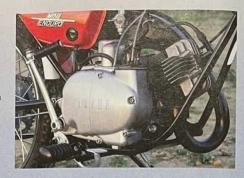
The Mini Enduro was not a technical tour de force. Its 58cc rotary-valve two-stroke single, fed by a tiny, 16mm Mikuni and lubricated by a no-fuss Autolube system, made very little power. But it was durable and reliable, and even after a long winter's nap in the Midwest or northern tier of the country, they'd fire right up come springtime — with a little help from leaded, non-ethanol fuel, of course.
