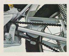
with fast throttle response is back-lash in the transmission and chain. YAMAHA has eliminated this problem on the TY80B by including a transmission with closer tolerances and installing a chain tensioner on the rear swing-arm. The chain tensioner maintains a constant tension on the chain at all times by taking up any chain slack that should occur.
