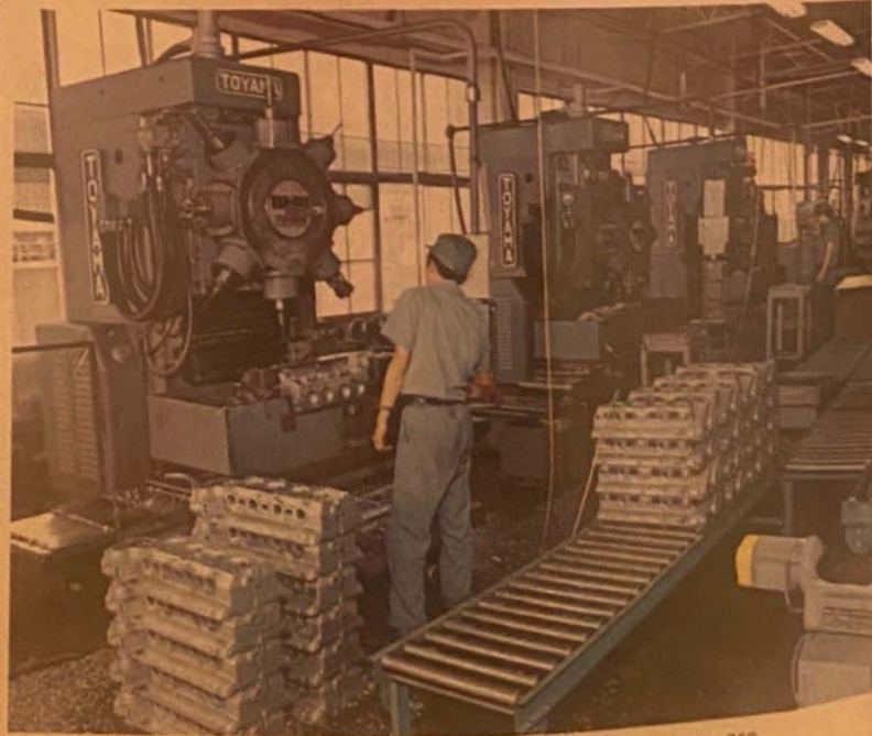
▲ "Machine tool shop: cylinder blocks for large scale engines are treated by special drill presses."
