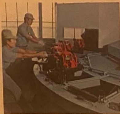
▲ "Tank test: while still inside the factory, completed motors are immersed in a water tank for final tests."
