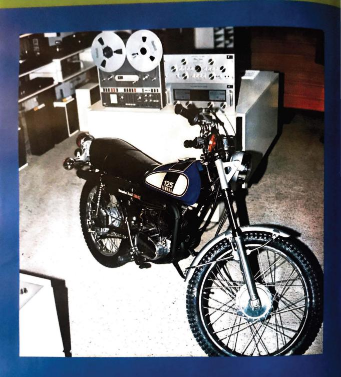
Emergency stop, slowing down; both can be done with equal confidence. Aluminium single leading shoe drumbrakes in front- and rearwheel give rapid heat-dissipation. The brakes are designed with double ridge scaling, ensuring they are water- and dust-proof under all conditions.
