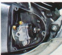
to be mixed with the gasoline. This is accomplished by precisely and continuously monitoring the engine speed and throttle opening so that only the exact amount of oil for optimum engine performance will be added. This system was developed in order to end the messy need for manually mixing the gasoline and oil, and as an extra benefit engine life is greatly lengthened because, the engine is always operating at optimum efficiency.
