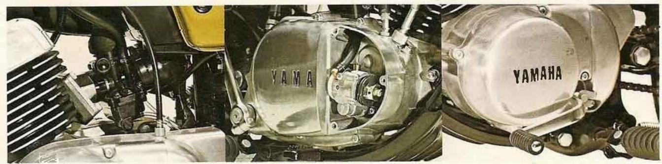
Torque Induction, Yamaha's unique intake system, utilizes a reed valve to feed the engine the exact amount of fuel and air it needs. The result is that horsepower is increased, particularly at low rpm's.
