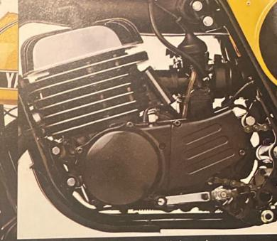
Omni-phase Balancer®-a special lightweight competition unit-cancels out engine vibration with a counterrotating balance driven off the crankshaft. The result is less fatigue to rider and machine.
