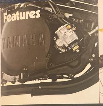
Autolube constantly adjusts the flow of oil into the fuel mixture according to engine load and speed, resulting in increased engine life. For those who want to save a little w and premix, the unit is easily detachable.
