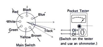
If the readings or the above six measurements are nearly  $\Omega\Omega$ , and no short-circuit is noticed between the terminals, as well as between the lead terminal and the switch body, the main switch is in good condition.
