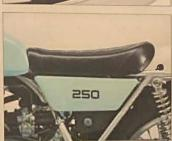
Silm trials saddle and narrow crankcase allow comfort, even when you're up on the pegs, and allow you to slip between obstacles.
