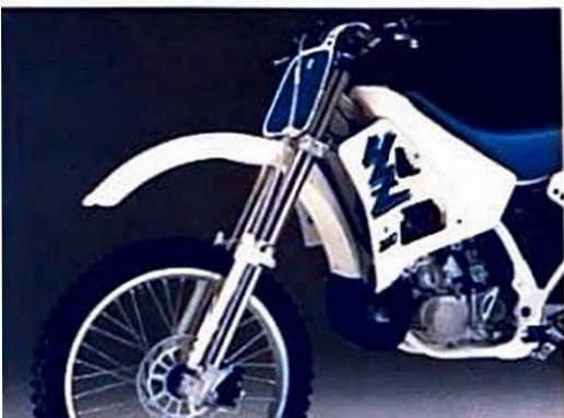
Works-style "upside-down" forks provide greater rigidity and fork tube clearance.
