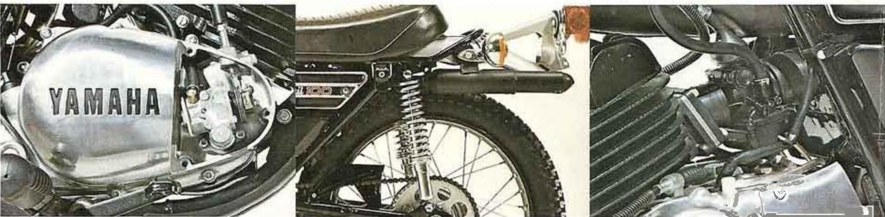
Autolube, a feature on all Yamaha twostroke engiens, automatically injects oil into the fuel mixture, eliminating the need for premixing. And, since it adjusts the flow of oil to engine load and speed, it extends engine life.
