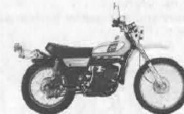
'75 model with a renewed fuel tank. Cylinder, cylinder head and crankcase are also redesigned.
