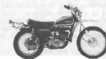
'73 model with a raised front fender and thermal flow rear suspension
