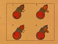
No pre-mixing of oil and gas is necessary. Both the gasoline and the oil are separately sent to the engine where they are regulated automatically and with extreme accuracy to supply exactly the correct mixture. Features: 'No gasoline/oil mixing 'Engine oil stays clean 'No engine overheating engine stays clean 'No smoke and no carbon \*Less engine trouble and longer service \*No troublesome engine adjustment...maintenance costs are lower \*Smooth starts and fast acceleration.
