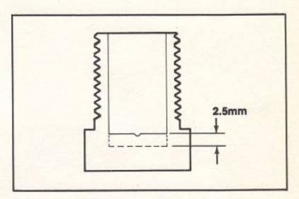
Note that the bottom of the hole has been machined flat; this must be done to avoid damage to the crankshaft.
