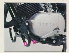
**Got-peg guards** (patent pending) For added protection under severe operating conditions, guards were installed low on the machine to protect the brake pedal, shift lever and the rider's feet from injury due to rocks and other obstacles.
