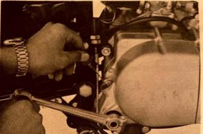
After draining the oil, fully tighten the oil drain bolt, and fill with new oil up to the specified level.
