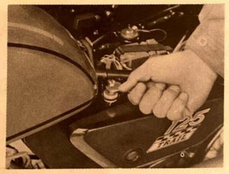
c) The cleaner element can be pulled out.
