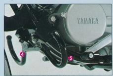
4 Foot-peg guards (patent pending) For added protection under severe operating conditions, guards were installed low on the machine to protect the brake pedal, shift lever and the rider's feet from injury due to rocks and other obstacles.
