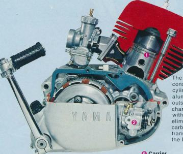
17-port Torque Induction Engine (patented)
