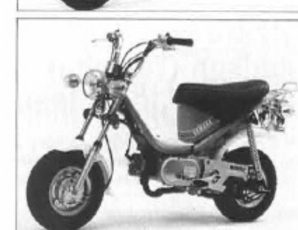
From top: The cycle styled Carrot MA50 (marketed in February of 1979), and the Towny MJ50 (marketed in February of this year). Both models have a shaft drive system.
