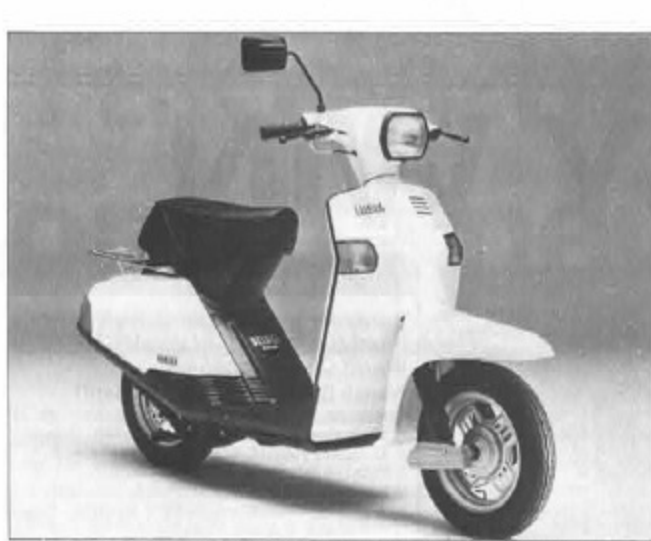
The Yamaha Beluga is a full-scale scooter which debuted as Yamaha's third stepthrough model in February of this year. The Beluga is oriented toward adult men who care about "quality". Its elegant styling and handsome meter panel are very favorably received by these customers. Available are the 50cc 3.8hp CV50E and the 80cc 5hp CV80E for pillion riding. Both have an electric starter and V-belt type automatic transmission. Both brakes are hand operated. The CV50E has 3.00-10-2PR tires and the CV80E 3.50-10-4PR ones. They weigh 75kg and 79kg respectively.
