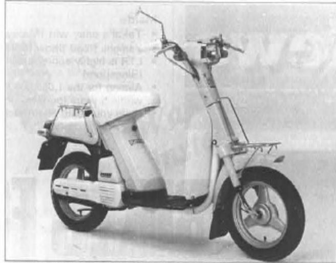
The Yamaha Passol S50 which was first marketed in March 1977 is noted for its exclusively gentle feel. Anybody in whatever costume can ride it with ease. It is an effective developer of market potential. Its step-through type chassis is another sales point. Handling ease also appeals greatly to women. The forced air-cooled 2-stroke 2.3hp engine is mounted under the seat. The rear wheel is driven by an oil-bath type chain through an automatic transmission. The automatic choke and C.D.I. system ensure positive kick starting. Both brakes are hand operated. Weight: 42kg, fuel consumption: 75km/lit. (30 km/h), Tire size: front & rear 2.50-10-4PR. The S50D has a fuel meter and oil meter.
