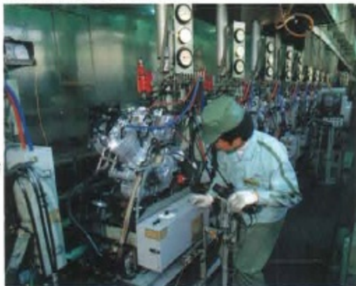
Yamaha's new power! V-twin XV750 and XV1000 (TR1) engines are taken one after another for final inspection.
