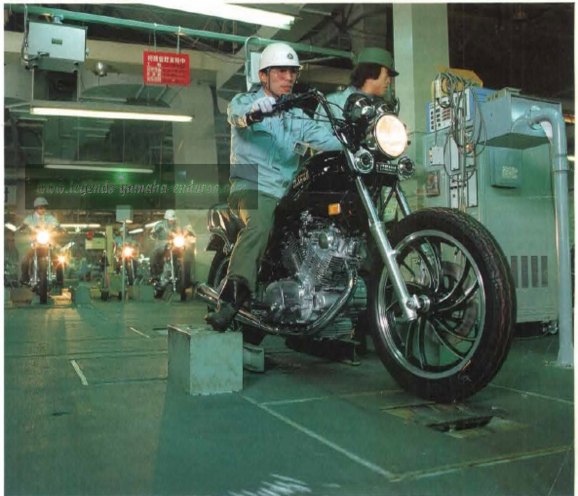
Firing test. The 75° V-twin engine and its unique exhaust. The capacitor discharge ignition system undergoes its final adjustment.
