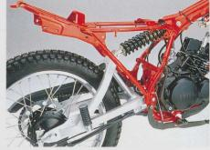
Yamaha's Monocross suspension was developed from the World Championship motocross, and combines good comfort with total control. The triangulated, box-section swinging arm adds extra rigidity to the chassis and ensures positive girp and confident handling. And the De Carbon type gas/oil shock absorber provides constant, reliable damping while allowing for a full 130mm of rear wheel travel.
