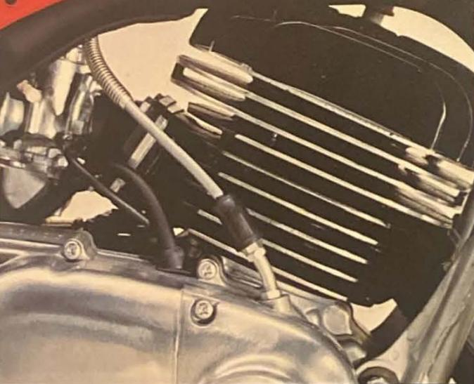
**Torque Induction.** Yamaha's exclusive reed-valve intake system, produces remarkable low-speed torque. The large flywheel engine and wide-ratio, six-speed transmission also help it pull hard at low speeds.
