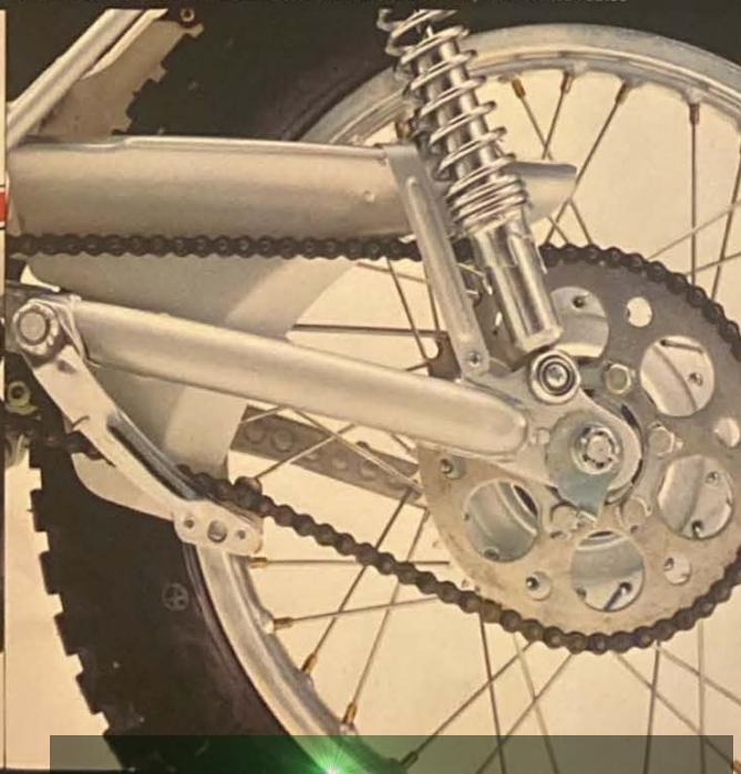
**Chain tensioner and oiler.** In order to prevent the chain from stretching when the engine is cold, a chain tensioner is attached to the rear swing arm to maintain a constant chain tension. Also, one side of the rear swing-arm is utilized as an oil reservoir.
