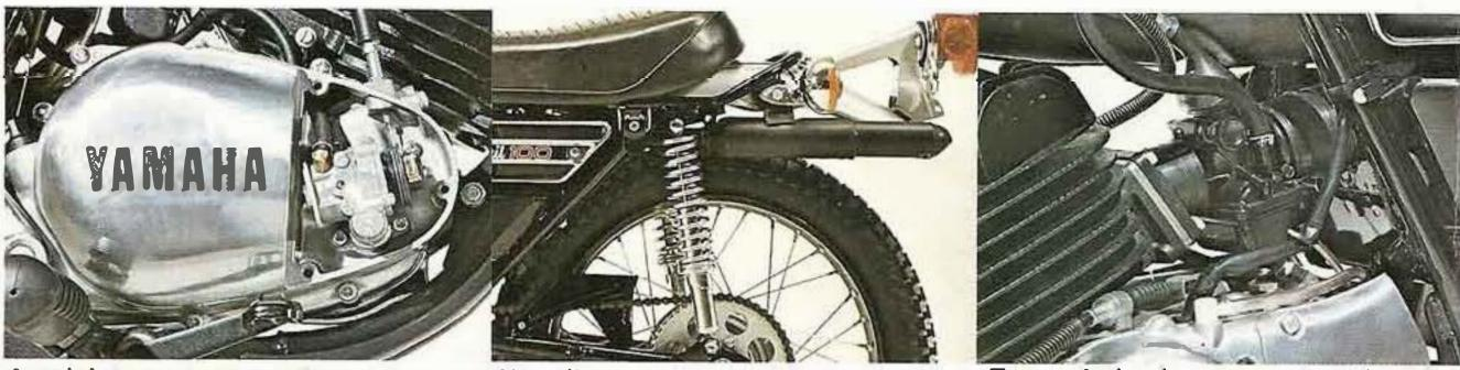
Autolube, a feature on all Yamaha twostroke engiens, automatically injects oil into the fuel mixture, eliminating the need for premixing. And, since it adjusts the flow of oil to engine load and speed, it extends engine life.
