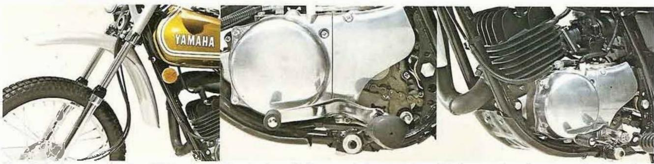
New high-clearance fender of lightweight polypropylene is virtually unbreakable. New front fork design and new steering geometry help 1974 Yamaha Trails handle like motocrossers on rough trails.
