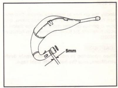
To align all items properly, tack weld the head pipe while it is in place on the motorcycle,
