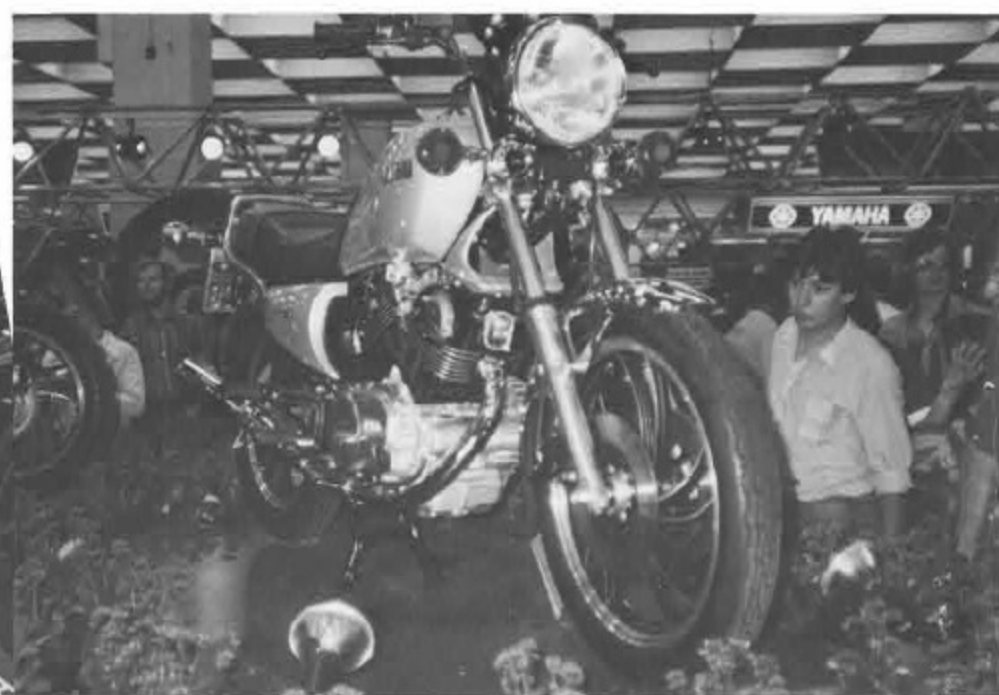
The TR1 (XV1000) features a very slim V-twin layout.
