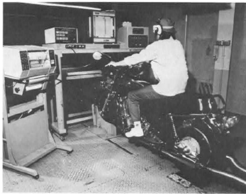
Exhaust emission test.
