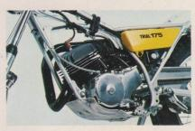
In order to assure that the TY175B will be able to withstand the severe treatment encountered on the roughest section, the frame design is a doublecradle type. This frame, with its hightensile-strength, tubular-steel construction, is based on the frames of the famous YAMAHA Motocross and Road Racer machines which have been consistent championship winners on leading
