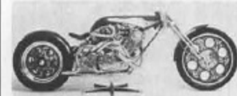
Reed's special XV1000 is truly a custom bike masterpiece. Virtually every component on the machine is handmade. All except the brake callipers, rear shock absorber, tyres and drive belt. Plus, of course, the Yamaha XV1000 engine!
