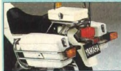
Document box and saddle bags: The optional document box (280 x 200 x 80 mm) and standard side saddle bags (415 x 145 x 270 mm) are made of ABS/SPCC plastic for rugged durability. Highly convenient for storage of paper work, equipment and tools.
