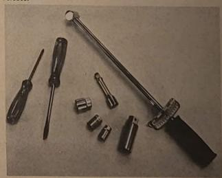
Installation of the Webco head, expansion chamber, and Filtron element air cleaner on either AT-1 or CT-1 requires only 10, 13, and 17mm sockets, a 3 inch extension and some sort of handle, a plug socket, torque wrench, Phillips and slotted head screwdrivers. Job can be done in two hours.
