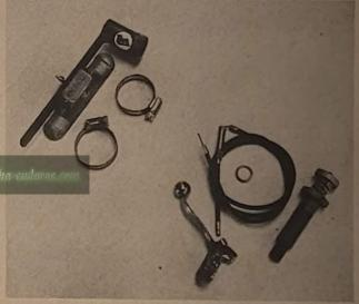
Webco has dozens of dirt-bike accessories including this holder for two spare spark plugs (left) and a compression release.
