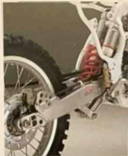
Deltabox swinging arm with Bilstein-type shock
