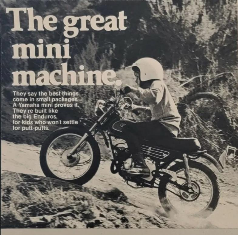
Now Yamaha makes two mini's: The JT2L-Mini Enduro with street-legal features and the snappy JT2-Mini MX, for off-road riding. Both bikes are built tough like the big Enduros, with full 15-inch spoke wheels, 60cc rotary-valve engine, Autolube oil injection, sure-stop brakes and a 4-speed constant mesh gearbox. They're both safety engineered from the ground up. You and your Dad should look them over. They're ready and rarin' to go at your Yamaha dealer.
