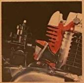
2. Exclusive Yamaha TORQUE INDUCTION<sup>®</sup> means better breathing and more horsepower at all rpm's. Reliable stainless steel reed valve between the carb and cylinder opens on engine demand, closes to prevent blow-back 7-port breathing means more power, cooler running.
