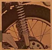
6. Double-spring, adjustable rear shock absorbers. One spring smooths out the vibration caused by minor roughness in the road while the other spring cushions the larger shocks. The overall tension may be adjusted to any one of five positions according to the roughness of the road
