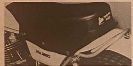
YPDI offers a longer seat on the same base style. Height of seat is only slightly increased while length is nearly doubled, padding increased. Seat offered by Malcolm Smith Distributing is snapped onto original base and has a whole bunch more padding. Two 10mm hex bolts found inside near top of shocks hold seat in place.
