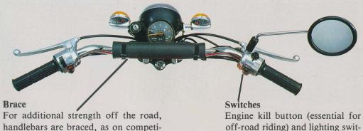
handlebars are braced, as on competition machines, and padded for rider protection.
