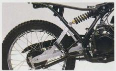
Yamaha's own Monocross suspension and its De Carbon type shock absorber.
