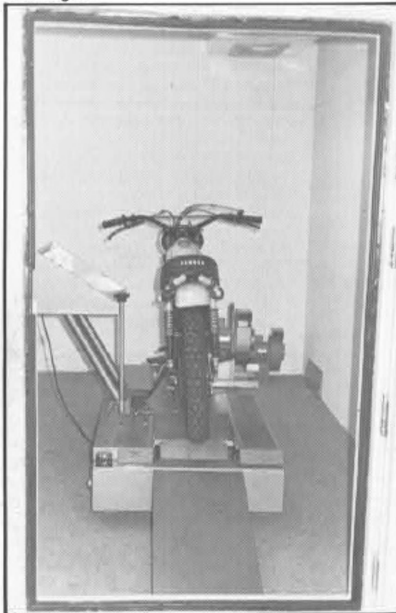
Bike lifts are made in Thailand and Japan. The tube seen on the right side is the exhaust system leading to an underground water tank. Each bike lift is fitted with this system. The tube is fitted to a muffler and switched on to prevent exhaust emissions from staying in the room while an engine is running. Exhaust emissions are induced and cleaned in the water tank, and then discharged.
