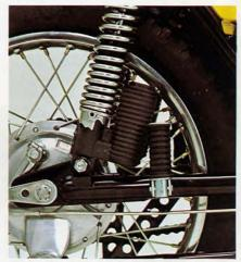
Thermal-Phase rear shock absorbers In order to maintain uniform shock-absorbing characteristics even when subjected to continuous rough riding, the rear shock absorbers are equipped with Thermal-Phase heat exchangers to cool the shock absorber oil keeping it at a constant viscosity. Also, the shocks are mounted slightly forward and at a greater angle to obtain a longer stroke, thereby improving road tracking ability.
