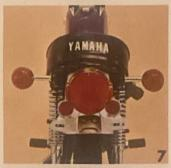
7. The stop lamp with extra reflectors yields positive recognition any time of day or night. The large stop lamp circuitry is so designed that the lamp will illuminate when either the hand brake or the foot brake are actuated and the headlight will not momentarily become dim.
