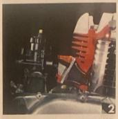
2. Yamaha's exclusive TORQUE INDUCTION® means better breathing and more horsepower at all rpm's. Reliable stainless steel reed valve between the carb and cylinder opens on engine demand, closes to prevent blow-back. 7-port breathing means more power, cooler running.
