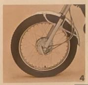
4. Enduro front forks are built to absorb shocks from the roughest roads while maintaining stability and maneuverability. The extra-large front brake has positive, dependable stopping action. It's designed to be water-and dust-proof for safe stops under any conditions. When the front brake is operated, the rear stop light illuminates, for extra safety.
