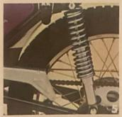
5. For maximum control and riding ease, the rear suspension is equipped with an adjustable 5 position are the rider to change the tension of the rear shocks.
