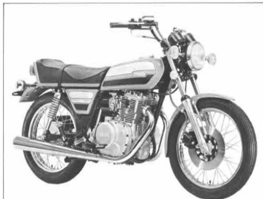
• 4-stroke OHC parallel twin engine, 66 x 52.4mm, 358.5cc • Compression ratio 8.7 : 1 • Max. torque 2.8-kg-m/7,500 rpm • Top speed 160km/h
