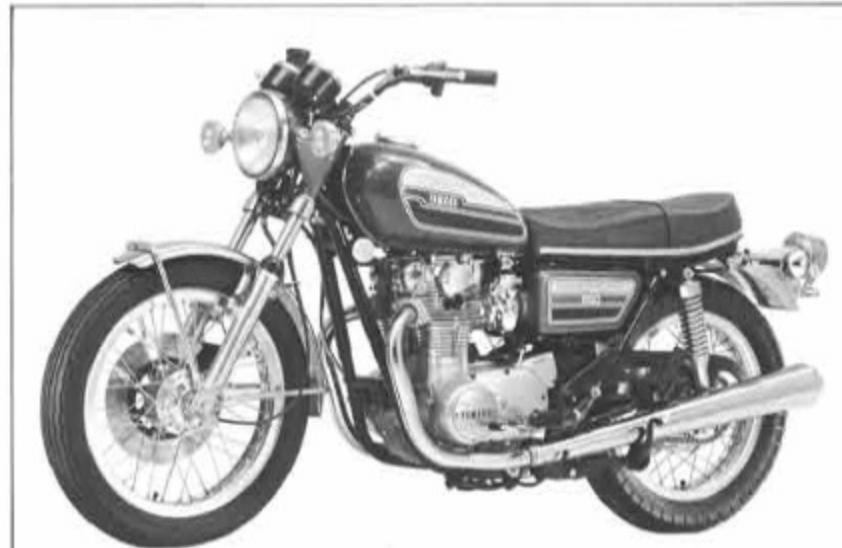
• 4-stroke OHC parallel twin engine, 75 x 84mm, 653cc • Compression ratio 8.4 : 1 • Max. torque 5.5-kg-m/6,000 rpm • Top speed 185 km/h plus
